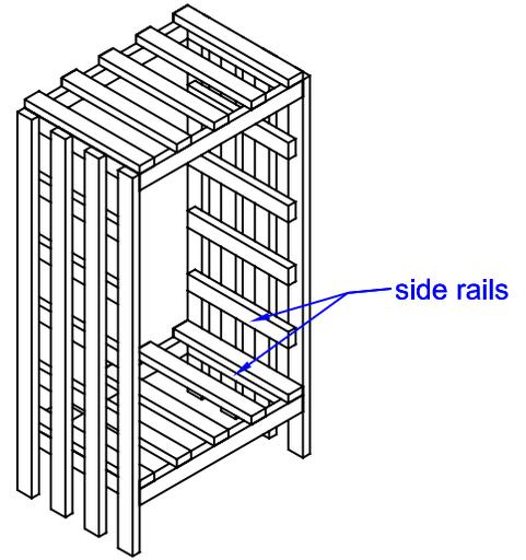
3. Keep adding shelves from the bottom up and nailing them on. Securing the top last.
